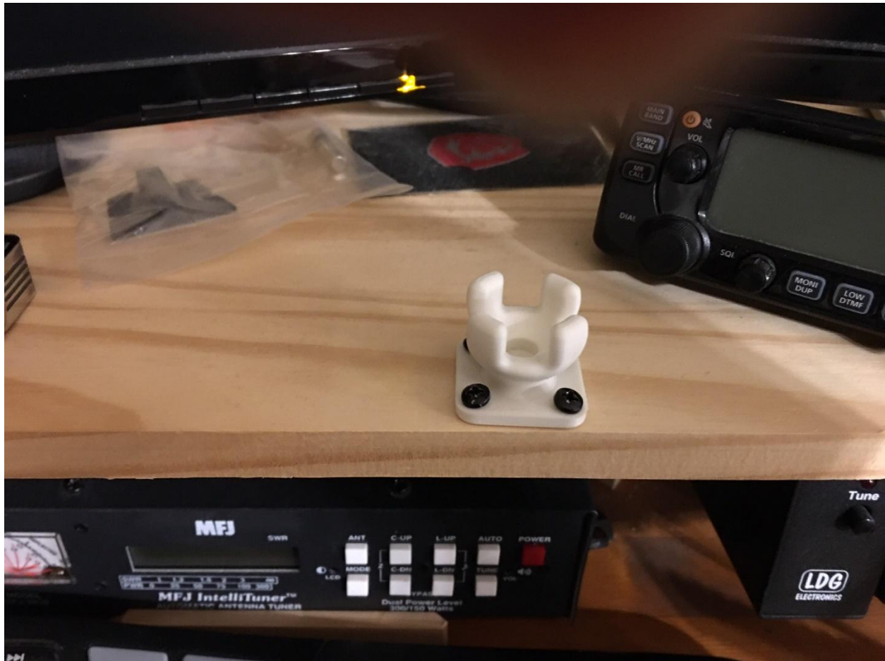
Exhibit 2: Socket mounted to my tiered shelf awaiting the control head with ball piece
