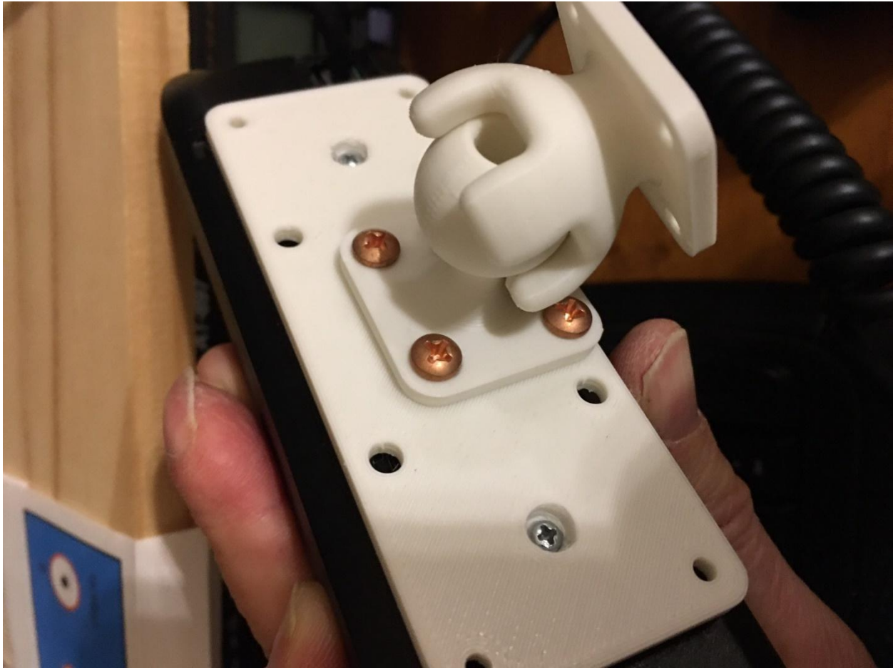
Exhibit 1: Test fitting backing plate with Ball and Socket mount on control head
